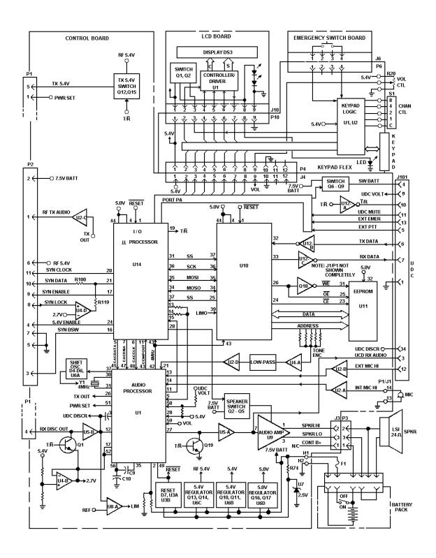
Figure 12 - Front Cover Assembly (Earlier) And Control Board Block Diagram
